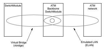
Figure 2-2 ATM Backbone SwitchModule Function
